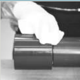
Cleaning and activation of the bonded surfaces is absolutely essential to ensure a reliable bond.
